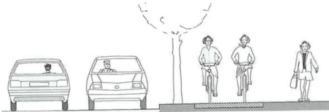
Figure 136. Schematic of an improved allocation of the limited Road Space to create cycling corridors
