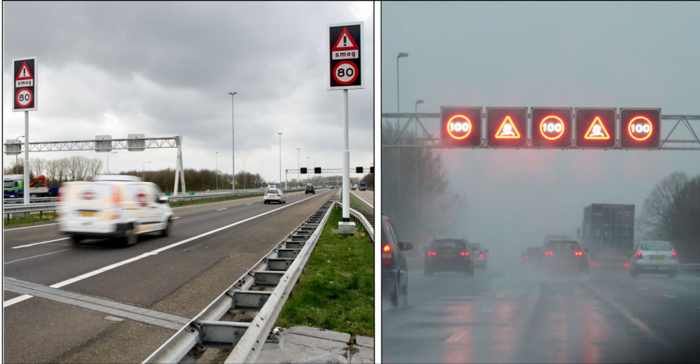
Figure: Rotation signs indicate a lower speed limit due to poor air quality on the A58 (left); Overhead matrix signs on the A12 Bodegraven – Woerden show a speed limit of 100 km/h as imposed in rainy circumstances (right).
