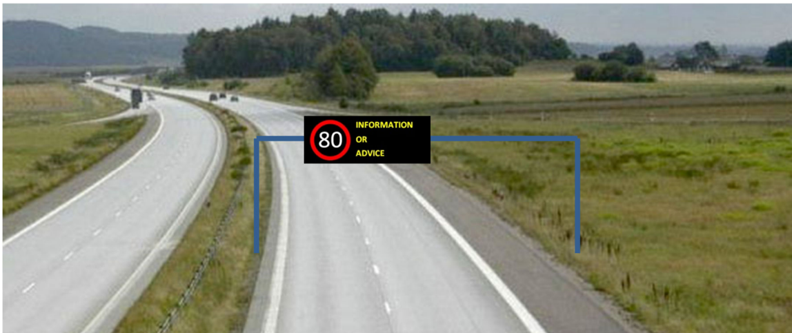
Figure 10: Portal mounted VSL signs on motorway, one speed limit sign integrated in VMS according to CL&FR5
