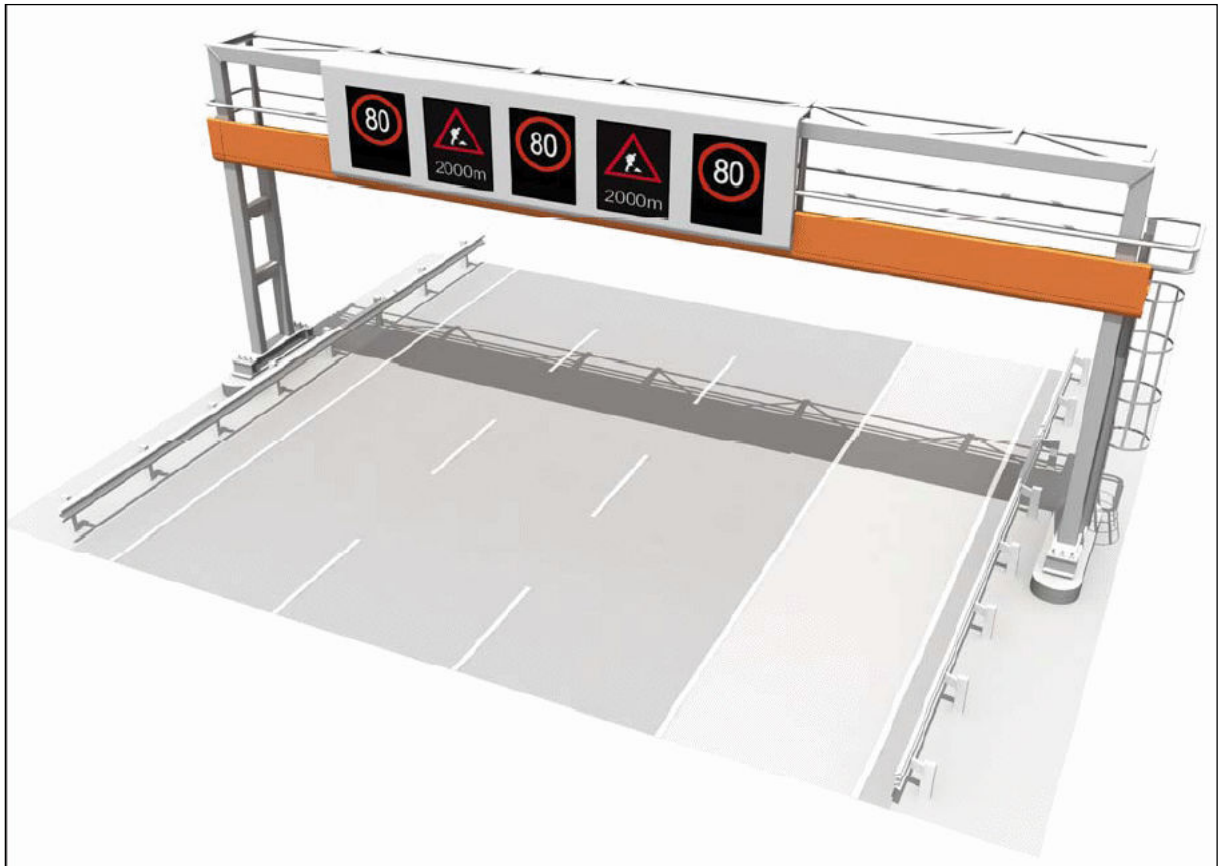
Figure 15: Example of an Austrian line control system with variable speed limits and warning signs on a common gantry
