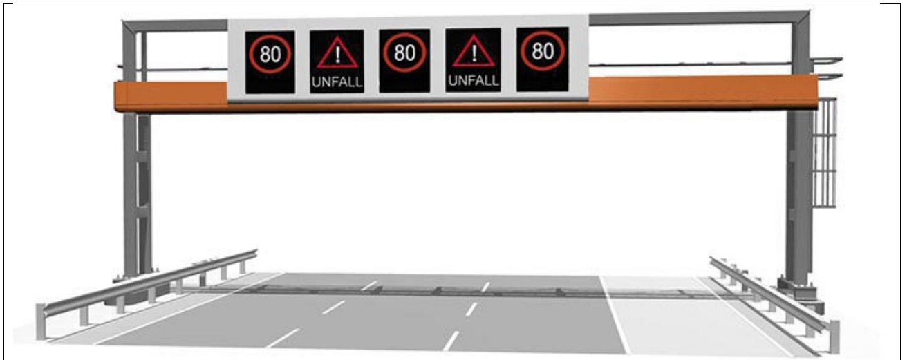
Figure 24: Example of an Austrian line control system with variable speed limits and warning signs on common gantry
