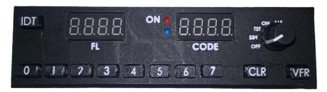
Pressing the 'IDENT' button highlights the aircraft's return on the surveillance display, enabling ATC to identify a particular aircraft. Only operate the function when instructed by ATC to 'squawk IDENT'.
