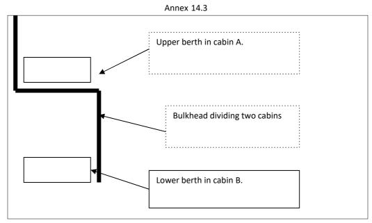
14.3.22.1 The horizontal width of the bunks shall be a minimum of 98cm. The saving in floor area is equivalent to approximately 50% of the bunk width. The drawback for such an arrangement is that cabins must be in line with one another, the plus point being that an area can be deducted from the width of a cabin (due to the overlap in bunk design) whilst still remaining close to the requirements of the MLC 2006.
