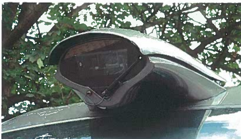
Plate 13: Civis' Optical Guidance Technology (Stagecoach has entered into an agreement with Siemens to develop similar technology on-board their existing fleet)
