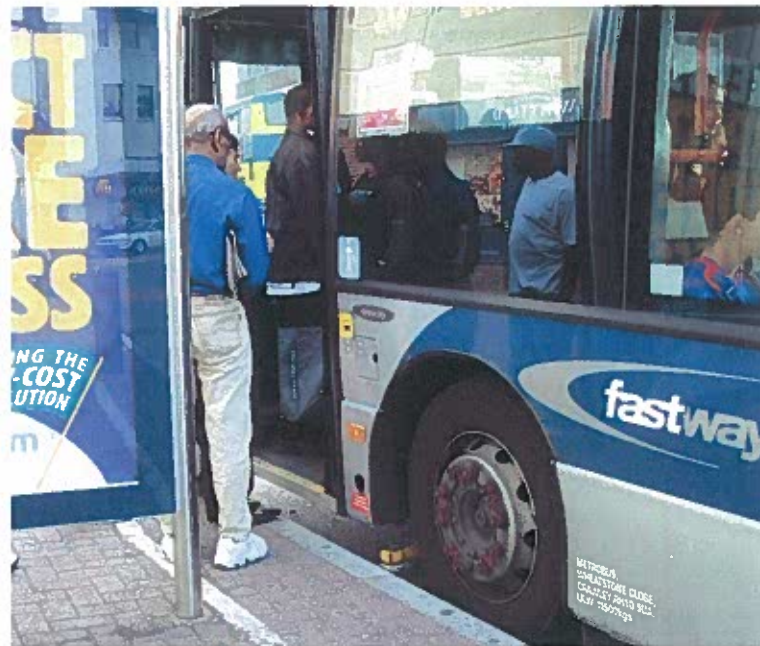
Plate 1: Kerb-guided bus docked at high kerb stop (guidance wheel and arm visible just ahead of tyre)
