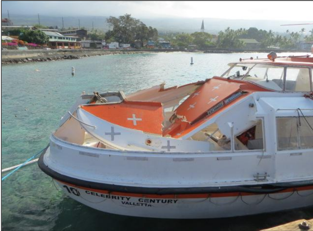
Figure 3A: Tender boat no. 10 - damage to upper structure
