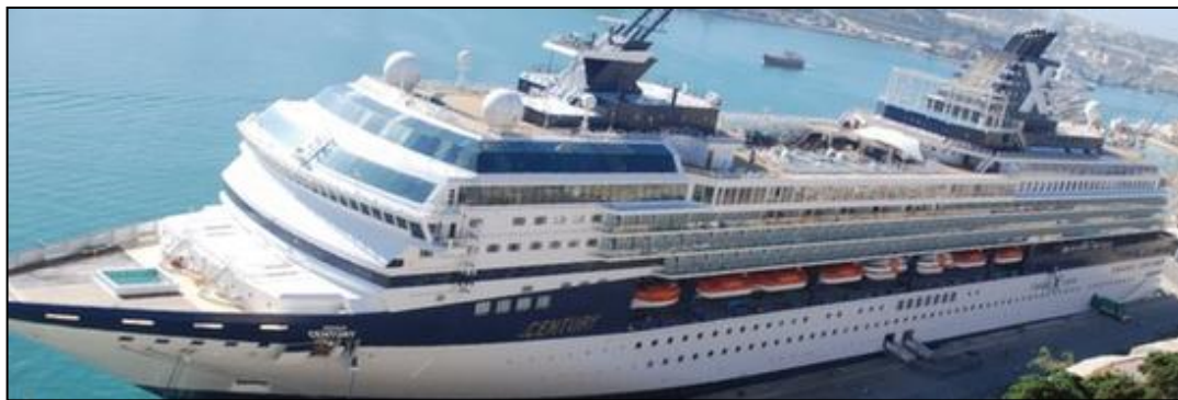
Figure 1: Celebrity Century 's port side, showing the location of the lifeboats and tender boats on Deck no. 6
