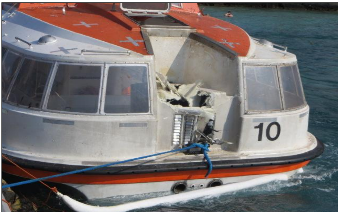
Figure 3B: Tender boat no. 10 - damage to the stern area from where the aft boat hook ripped out
