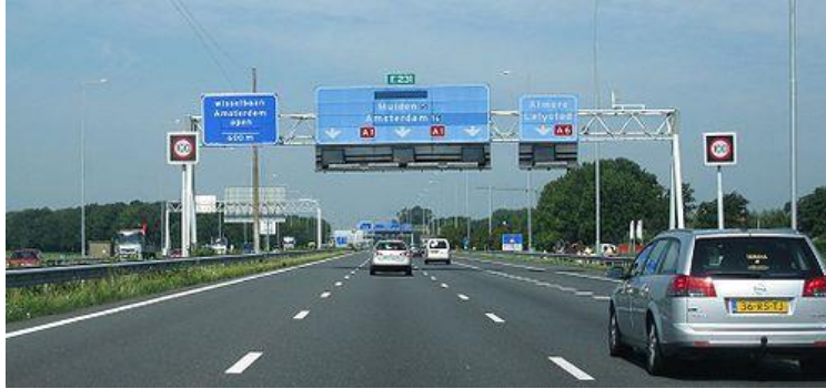
Figure 16: Entrance nr. 3 with dynamic route sign (median side). Tidal flow lanes open.
