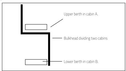
The horizontal width of the bunks shall be a minimum of 98cm. The saving in floor area is equivalent to approximately 50% of the bunk width. The drawback for such an arrangement is that cabins must be in line with one another, the plus point being that an area can be deducted from the width of a cabin (due to the overlap in bunk design) whilst still remaining close to the requirements of the MLC 2006.
