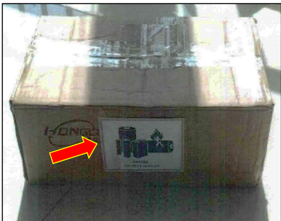
Figure 5: One sample package marked with the lithium battery mark
