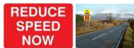
Figure 9: Warning sign indicating reduction in speed necessary for a change of road layout ahead
